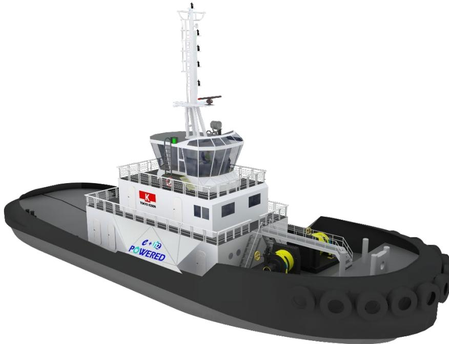
Tokyo Kisen Co., Ltd. and e5 Lab Inc. have jointly developed the new concept design of “e5 Tug,” electric propulsion harbor tugboat powered by large-capacity battery and a hydrogen fuel cell.
