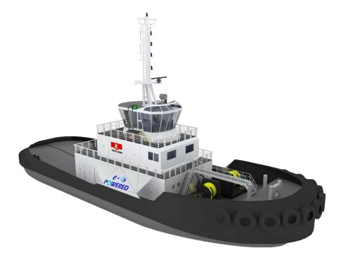
Tokyo Kisen Co., Ltd. and e5 Lab Inc. have jointly developed the new concept design of "e5 Tug," electric propulsion harbor tugboat powered by large-capacity battery and a hydrogen fuel cell.
